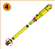
Screw the threaded pipe between the pump and the foot valve (P/N 0E10/20)
