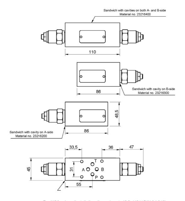
For NG6 valves (Installation dimensions to ISO 4401/ DIN 24 340)
