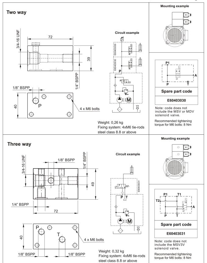
Note: 3/4-16 UNF manifolds can be stacked one upon the other but cannot be used with cetop 3 modular manifolds since the tie rods bolt pattern is different. The three way block is not compatible with square vertical tanks.
