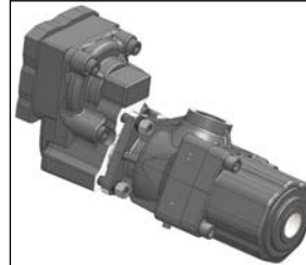
3 - Screw the nuts a few mm.
