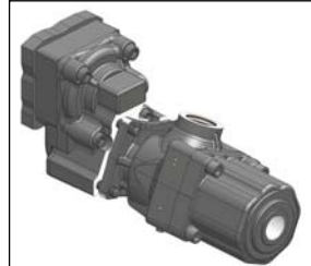
2 - Move the pump away from the PTO by 10mm.
