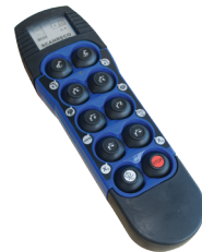
Handy 10-LCD can be supplied with one step, two step or with stepless infinitely variable (proportional) speed, and a graphic display for indication of value/icons from the crane/machine.
