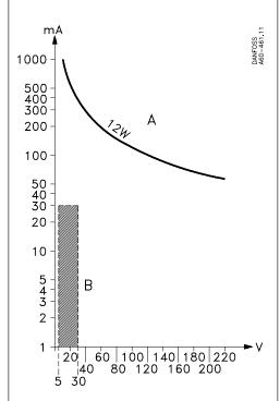
Curve A gives the maximum load. Hatched area B: Acceptable load for the gold plating of the contact.
